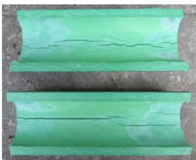
Dr Ingham explains "From a detailed examination of the fracture surfaces using optical and scanning electron microscopy and consideration of the operating conditions, it was considered that the cracking may have been caused by oxidative degradation of the polypropylene by the type disinfectant used in the pipe system. This hypothesis was confirmed by conducting oxidation induction time
